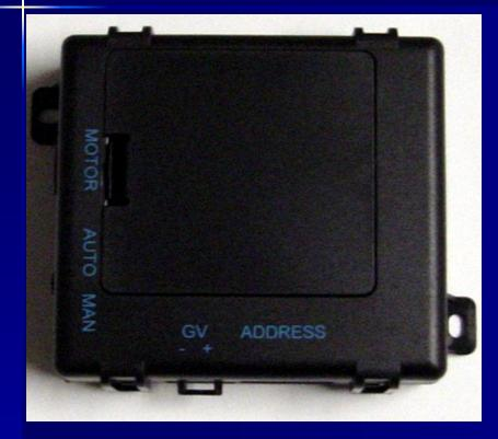
Connects to gas valve stepper motor to control BTU output.
