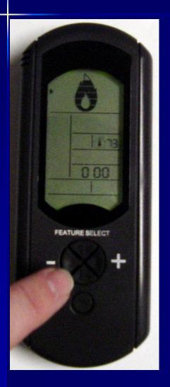
Allows adjustment of BTU output (flame height)
